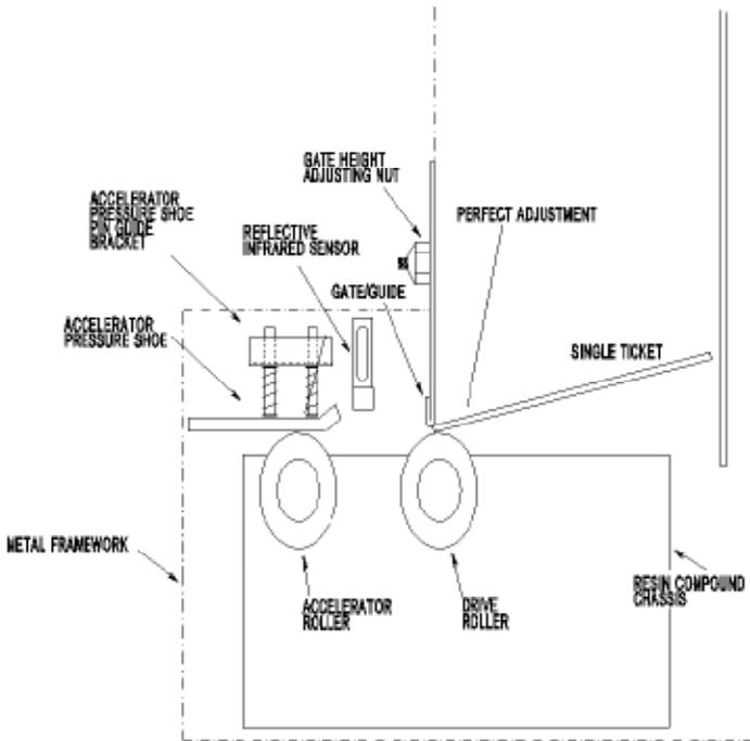
2. Adjust upwards for thicker tickets. Adjust downwards for thinner tickets.
