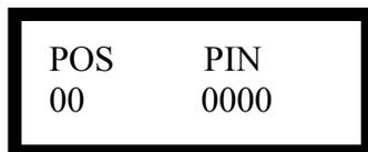
**To add or change a PIN number press \***. NEW PIN displays. Enter the new PIN number or enter 0000 to delete a PIN number for that position. Press the # key to advance to the next position. After you modify the PIN number, press the # key. When you reach the last PIN position, the display returns to the Main Menu.
