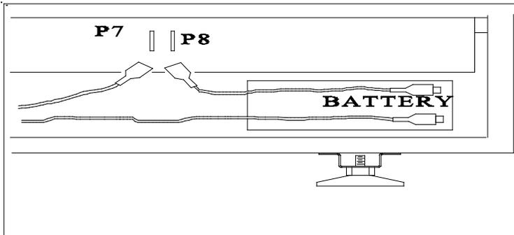
Plug in the two connectors as illustrated. The display on the console will now read ALARM ACTIVATED ENTER PIN NUMBER.
