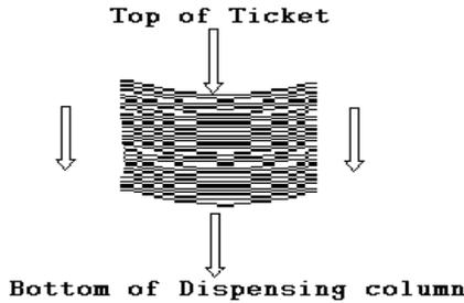
A wide opening at the top of each column allows you to enter stacks of tickets. Grasp a manageable stack of tickets. Slide the stack down the chute. Continue to load tickets until the column is full.
