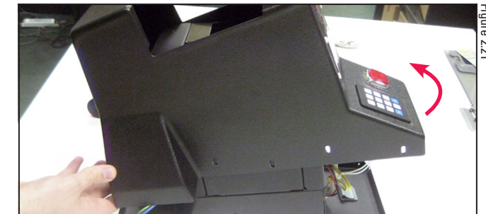
Use this motion to lift the plastic body
