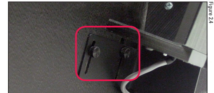
Notice the angle of the thumb nuts
