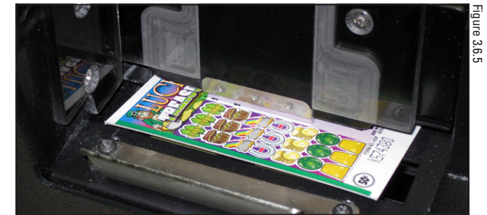
Place a ticket underneath the ticket gate
