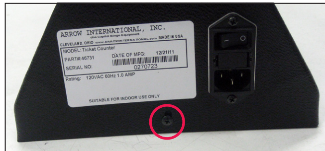
Remove this screw in the back as well
