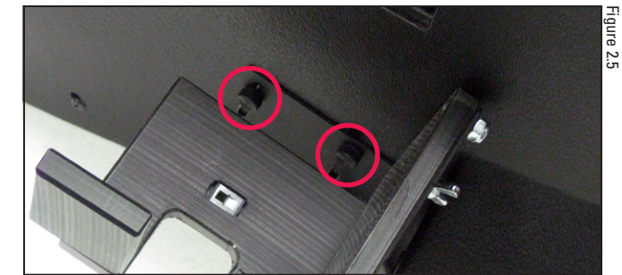
Remove the two thumb nuts
